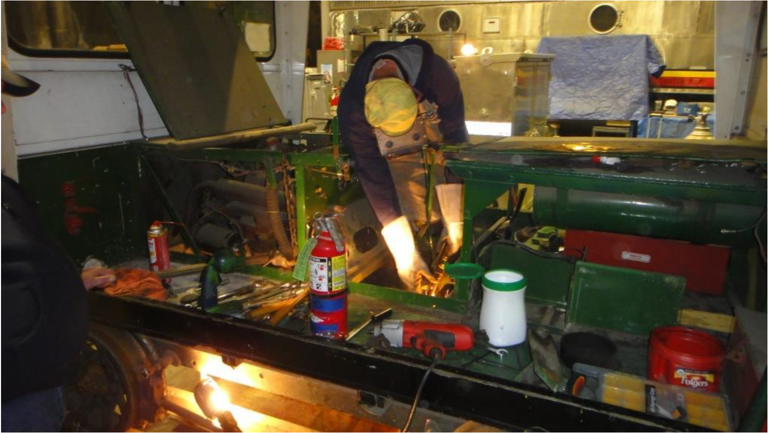
Cliff cuts the bracket holing the transmission in place on the A-4
